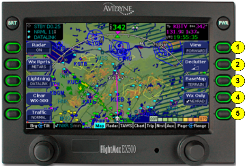
Figure 3.4 Map Page on 250nm Range with Forward View and "Terrain" base map.
